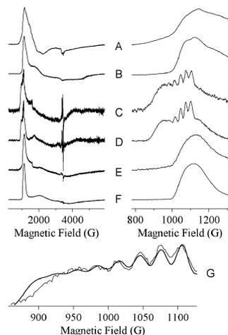
**Figure 2.** EPR spectra of 1 mM Co–VanX in the resting state (A, B), after 10 ms reaction with 5 mM D-ala-D-ala (C, D), and after complete reaction with D-ala-D-ala (E, F). The traces in G show the hyperfine region of spectrum C with a simulation overlaid indicating  $A^{\parallel} = 7/2(^{59}\text{Co}) = 3.5 \times 10^{-3} \text{ cm}^{-1}$  (33 G). Spectra A, C, E, and G were recorded at 9.63 GHz, 11 K, 2 mW; B, D, and F were recorded at 5 K, 200 mW.
